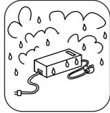
If the AC adaptor is used in steamy, damp, or dusty areas, it can cause a fire or electric shock.
